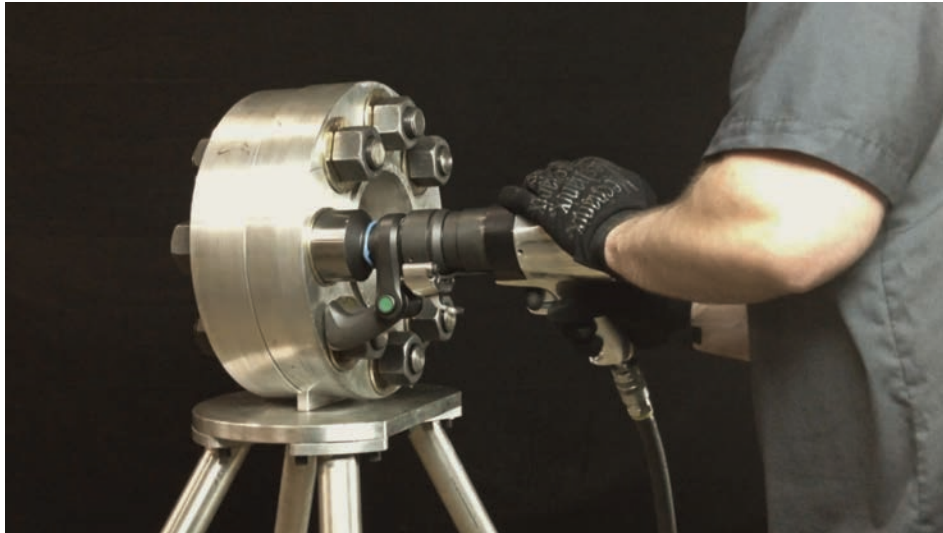
Figure 5 - Safety Position for THRILL Gun in Maximum Torque Setting
