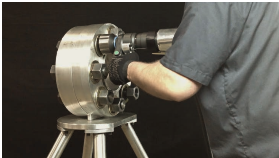
Figure 4 - Holding the THRILL Gun in the High Speed (Impact) Setting
