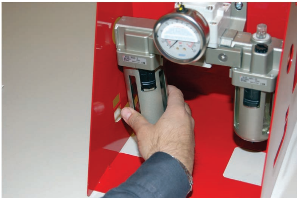
Figure 11 - Detaching FRL Reservoir
