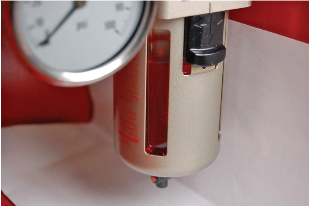
Figure 12 - FRL Unit, Lubricator 2/3rds Full of Oil
