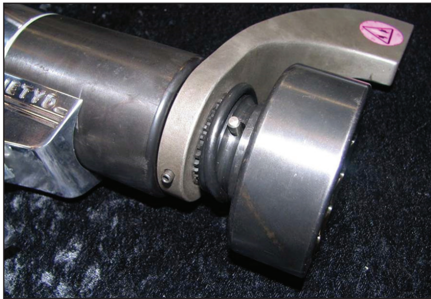
Figure 7. Installing Socket Locking Pin and Retaining Ring
