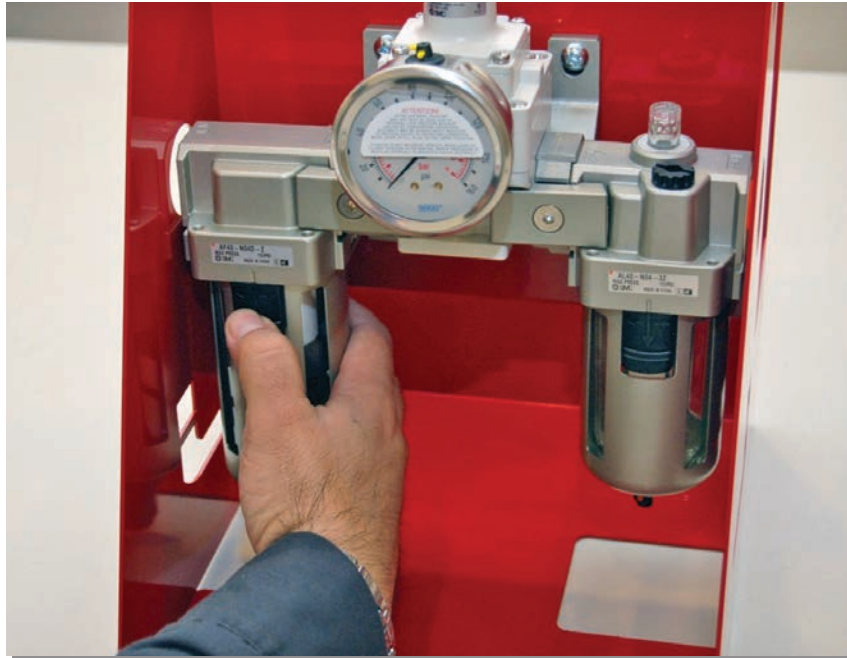
Figure 15. Emptying the FRL Filter Reservoir
