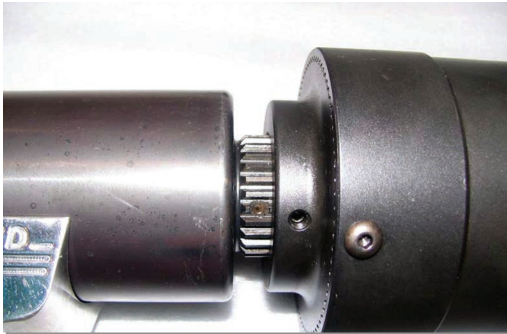
Figure 23. Aligning HYTORC Washer™ Socket Set Screw with Machined Recess in jGun Splines
