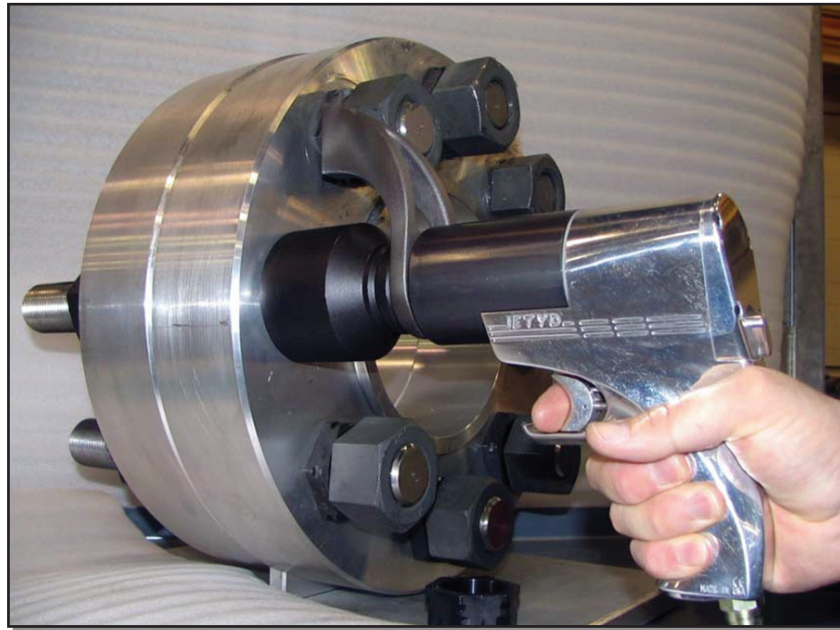
Figure 11. Using the jGun with a Reaction Washer
