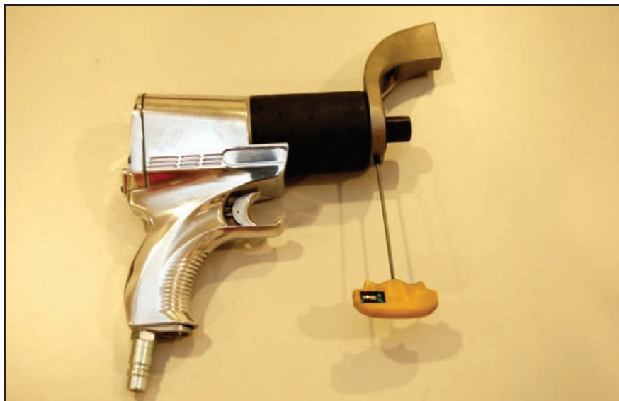
Figure 5. Tightening Reaction Arm Set Screw
