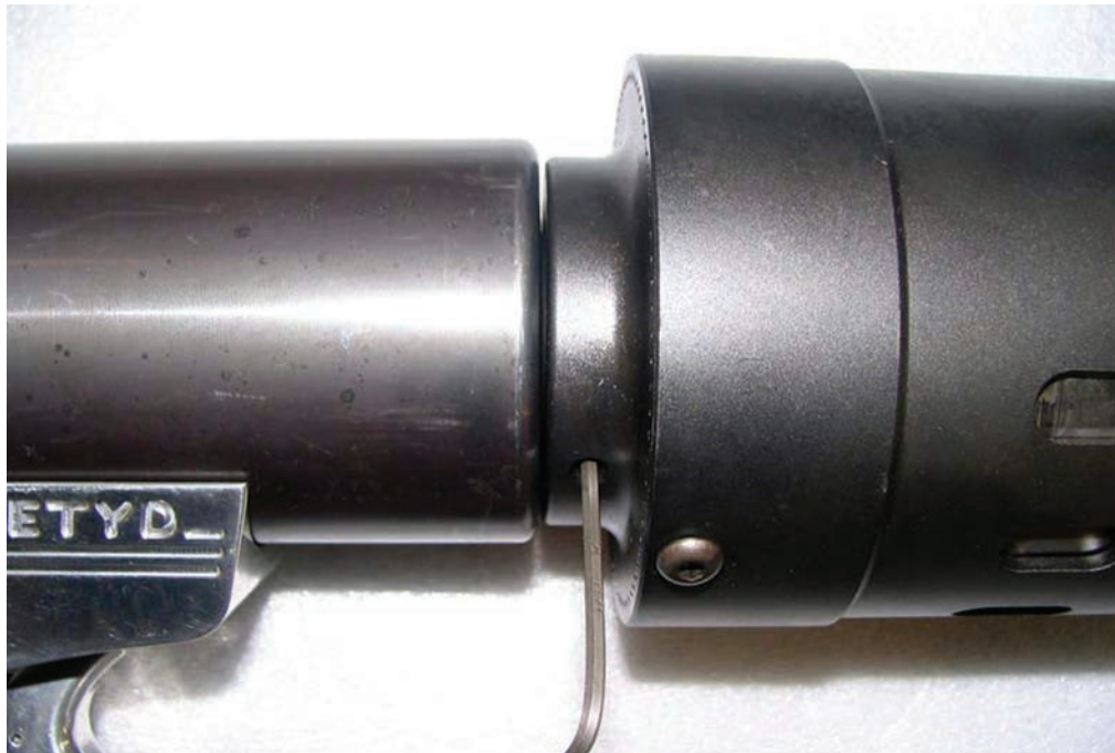
Figure 24. Tightening HYTORC Washer™ Set Screw
