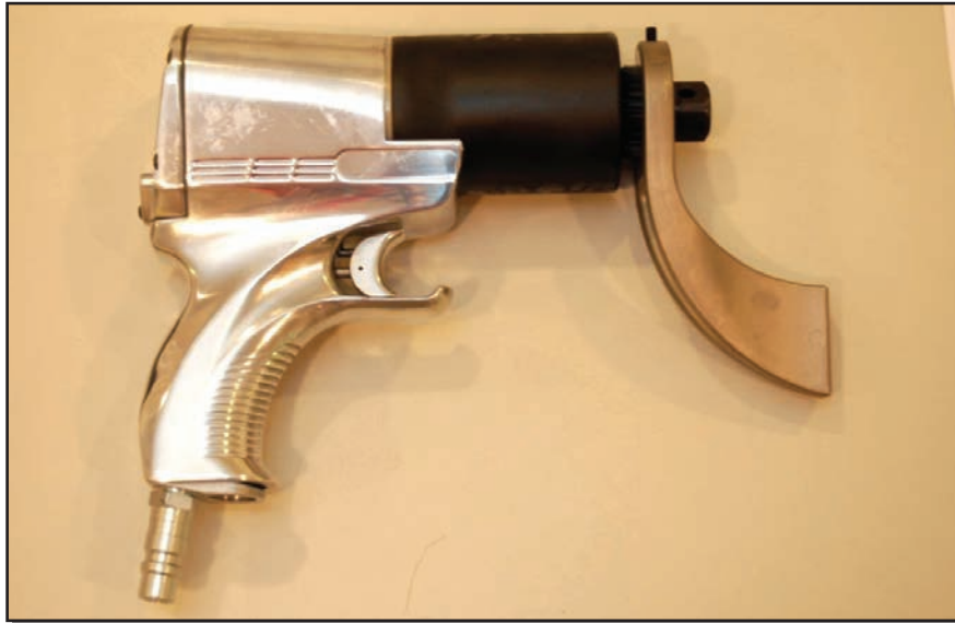
Figure 4. Reaction Arm installed
