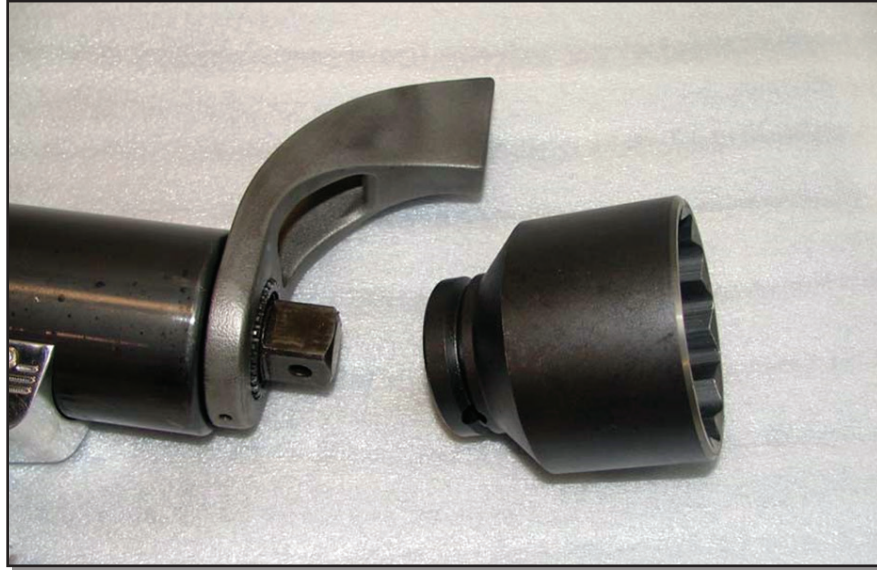
Figure 6. Installing jGun Socket
