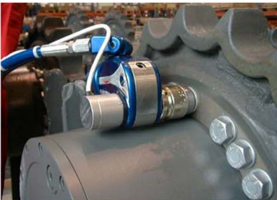
MXT-3 for the assembly of a caterpillar drive, according to the selected rotating angle
