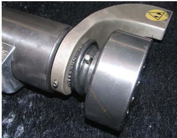
Figure 7: Socket Drive Attachment
