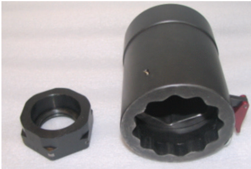
Figure 15: HYTORC Washer and Drive
