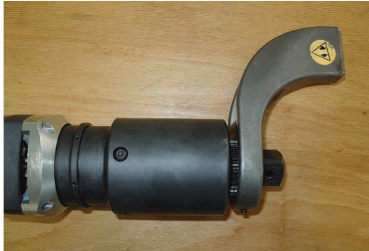
Figure 4: Reaction Arm Attachment
