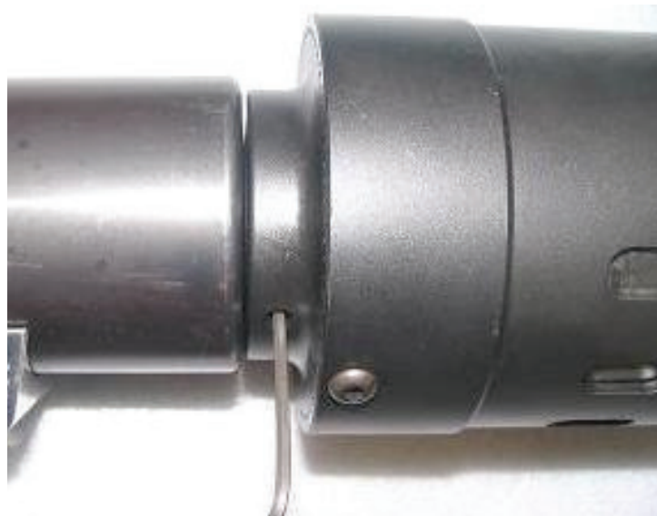
Figure 18: Tighten set screw
