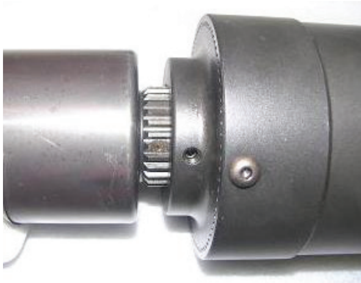
Figure 17: Installing Set Screw on HYTORC Washer Drive
