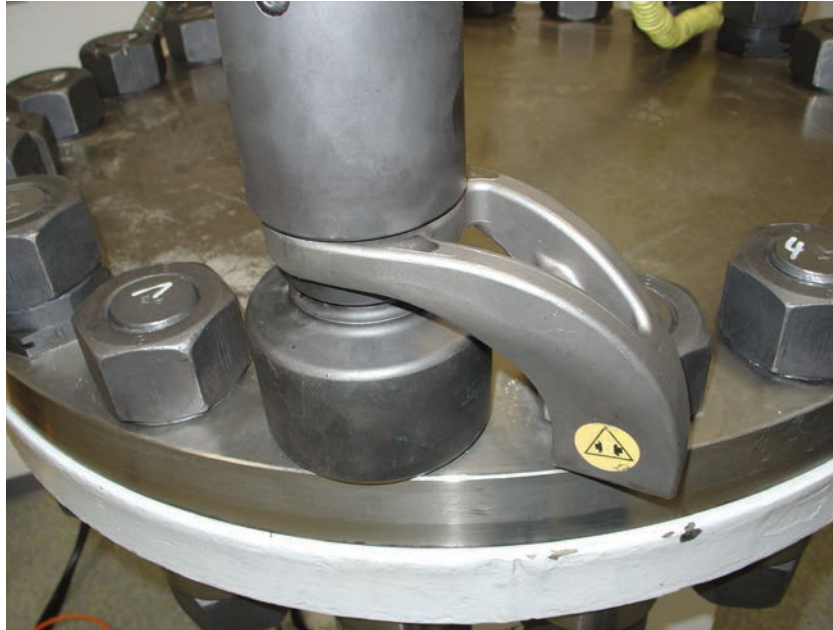
Figure 8: Reaction Arm Positioning
