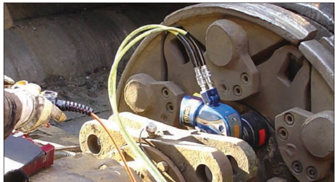
MXT-10 being used on a scrap press
