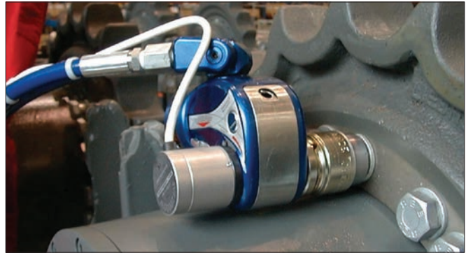
MXT-3 for the assembly of a caterpillar drive, according to the selected rotating angle
