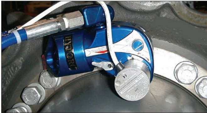
MXT-3 for the assembly of a caterpillar drive, according to the selected rotating angle
