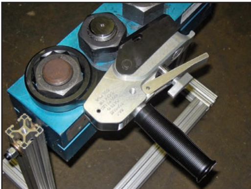
When loosening, the reaction foot will be located on the left side of the handle.
