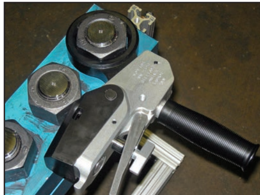
When tightening, the reaction foot will be located on the right hand side of the handle.
