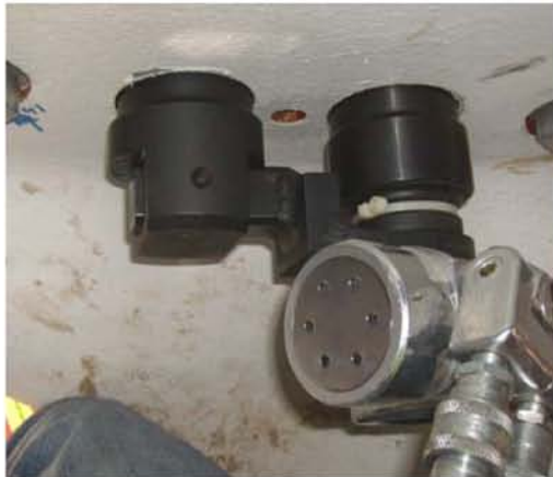
AVANTI-3 with Wind Cup Reaction Fixture
