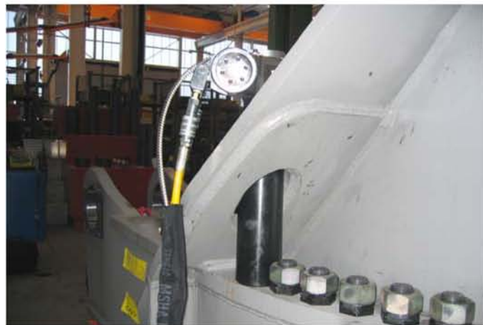
AVANTI-5 with side-load-free axial extension
